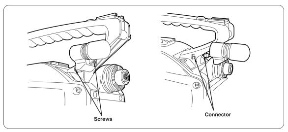
Remove the two screws to remove the connector and then remove the microphone.
